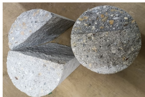
FIGURE 1. Horizontal construction joint during concreting (the core on the left disintegrated by itself upon removal from the structure).
