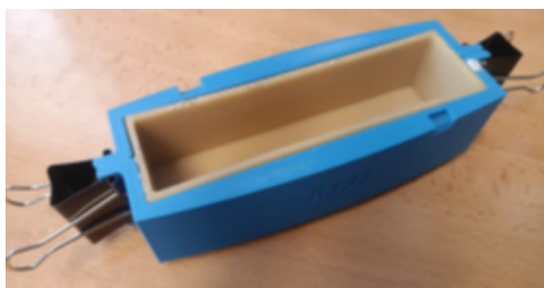
FIGURE 8. 3D printed mold with silicone insert.
