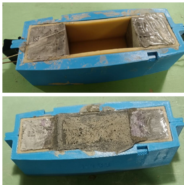
FIGURE 11. Top: first phase of pouring – older side parts of the sample. Bottom: second phase of pouring – complete sample with cast inner (younger) part.
