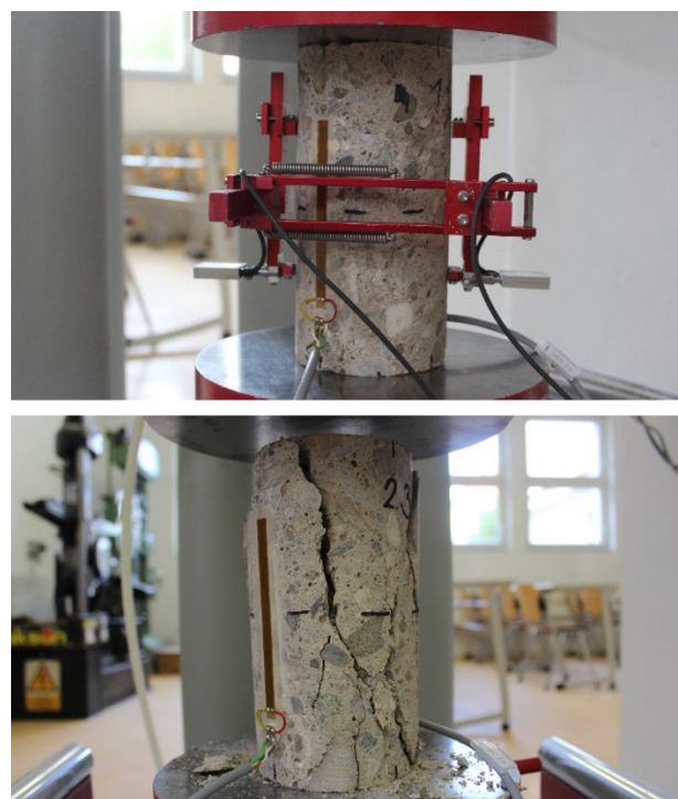
FIGURE 5. Test specimen during cyclic loading with strain gauges and extensometer (top), test specimen after failure (bottom).
