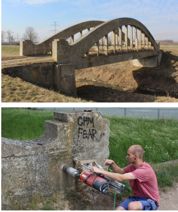
FIGURE 1. Arch bridge over Litava stream subjected to assessment (top), collecting of the concrete samples with the use of the core-drilling method (bottom).
