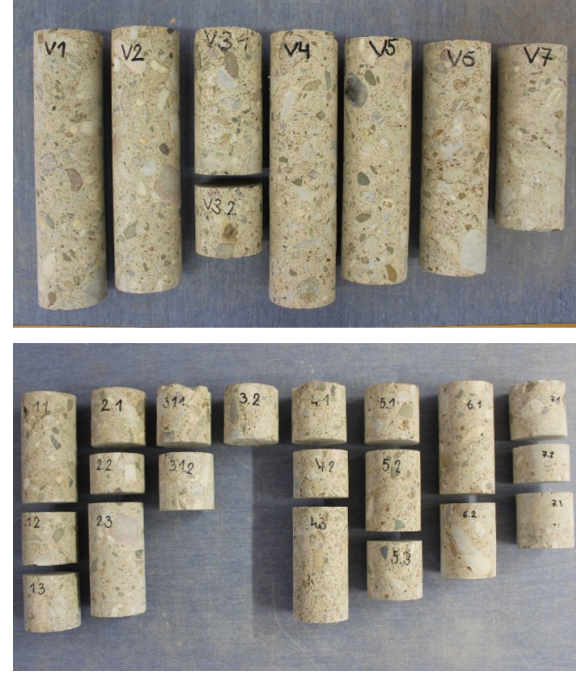
FIGURE 2. Core samples prepared for preliminary non-destructive sorting (top), cores divided into test specimens based on the results of non-destructive testing (bottom).
