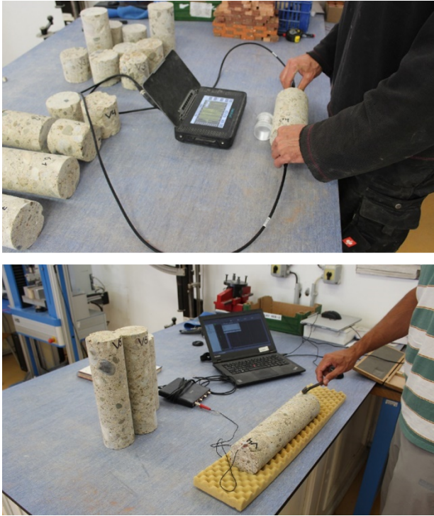
FIGURE 3. Non-destructive evaluation of the concrete samples and specimens. Ultrasonic pulse velocity method (top), resonance frequency method (bottom).
