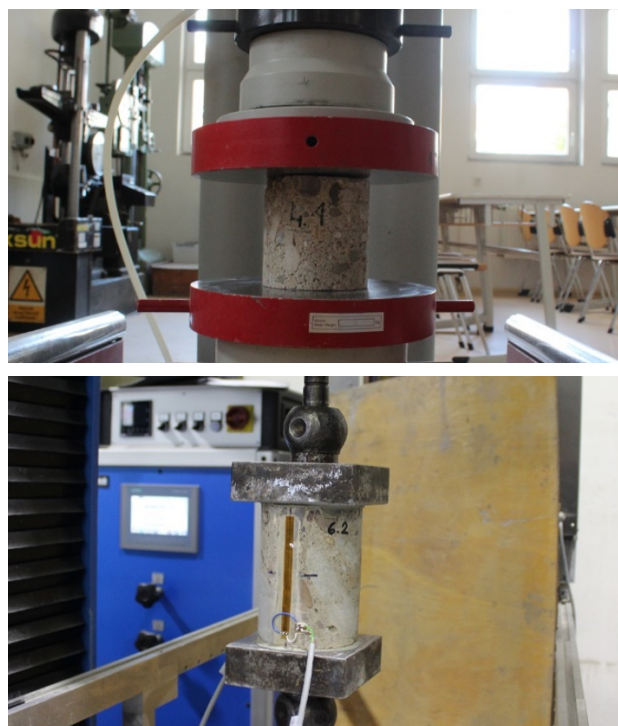
FIGURE 4. Compressive strength test (top), uniaxial tensile strength test with measurement of strain during the test (bottom).
