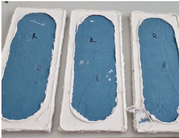
FIGURE 6. Specimens removed from the measuring device, sealant visible around the perimeter.
