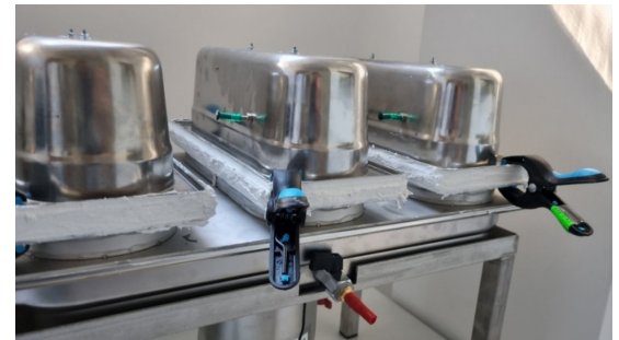
FIGURE 4. Measuring device with inserted and sealed specimens.
