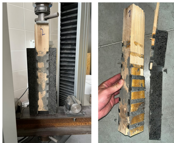
FIGURE 3. Comparison of results for the softwood – influence of ribs on the shear strength (left) and view of the sample SOF 11 before (middle) and after the loading test (right).
