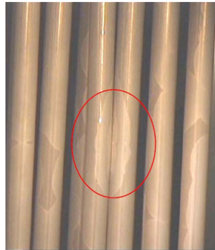
FIGURE 5. Rod bowing with rod-to-rod contact [5].
