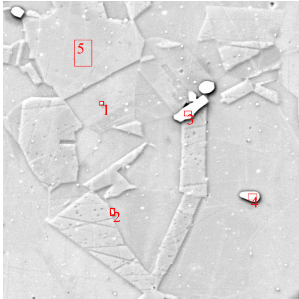
FIGURE 7. Areas of SEM-EDS analysis of specimen after high-temperature exposure at 1 100 °C.
