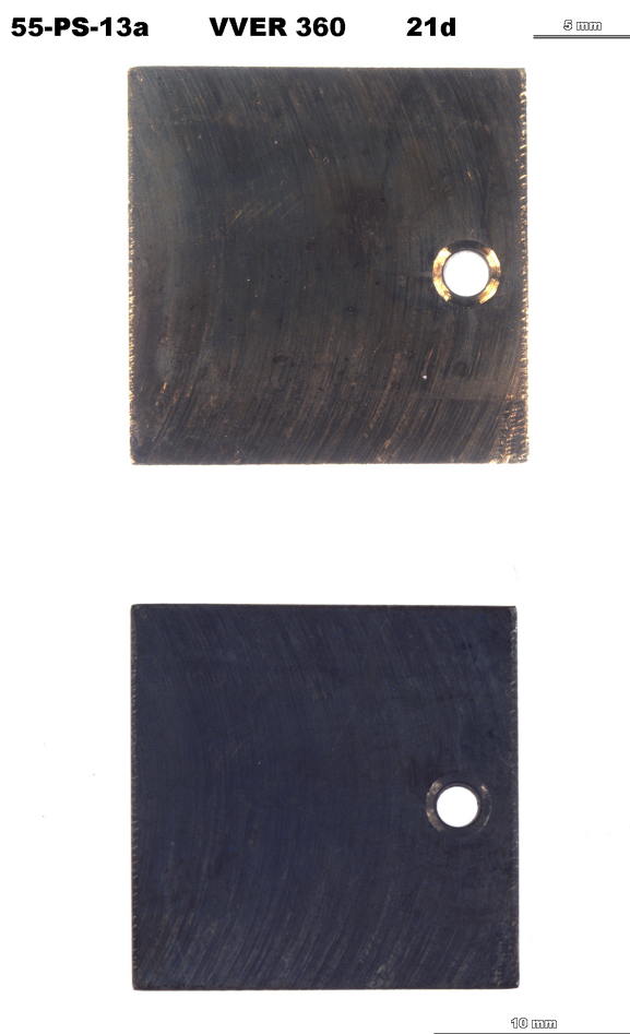
FIGURE 3. Pictures of the same specimen from the same side after 21 days (top) and 1659 days (bottom) of exposure in the WWER environment.
