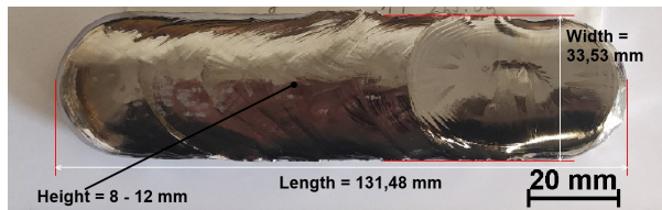
FIGURE 5. Geometry and dimensions of an arc-melted Zr-8Fe-8Cu ingot.
