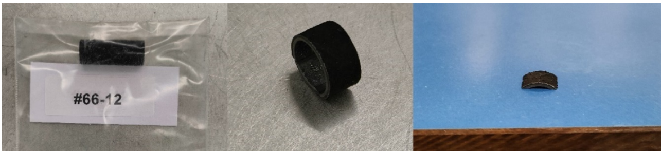
FIGURE 2. Preparation of SiC samples: on the left, the supplied specimen; in the center, the cut segments; and on the right, the final sample prepared for laser flash analysis.
