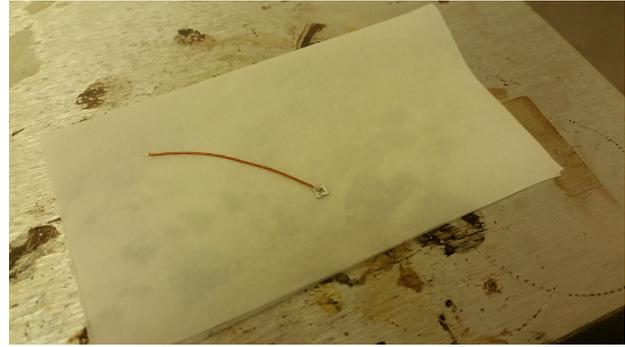
FIGURE 9. The diamond detector with wire glued to the electrode by silver resin (first detector)
