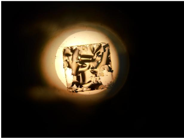
FIGURE 11. Delaminating layer on the second detector
