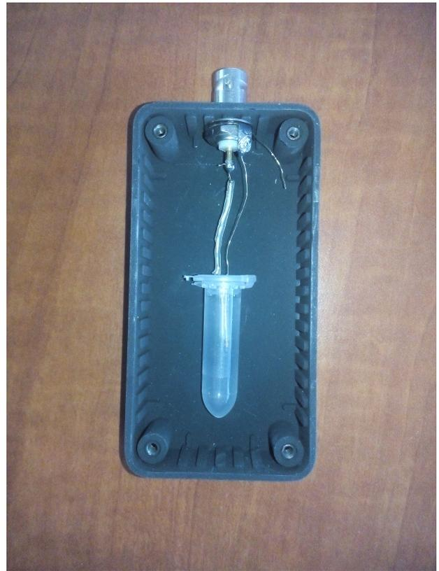
FIGURE 12. The detector inside the boron plastic box (the third detector)
