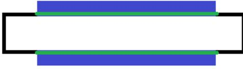
FIGURE 1. Diamond detector: diamond crystal (white), electrodes (green), conversion layer (blue).
