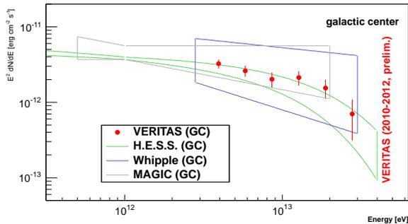
**Figure 1:** VERITAS energy spectrum measured from the direction of the GC (statistical errors only). Also shown are bow ties representing the spectra measured by Whipple [7], H.E.S.S. [8], and MAGIC [10].
