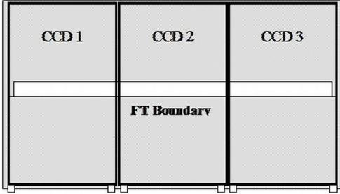
**Figure 3:** Schematic showing the region on the CCD where time resolved RSS spectra are recorded using a focal plane mask together with the spectrograph slit. Spectra of the target and sky are obtained in the rectangular region, which shuffled down across the frame transfer boundary at the end of a short exposure.
