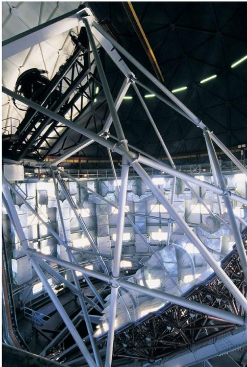
**Figure 1:** The 11-m Southern African Large Telescope (SALT), consisting of  $91 \times 1.2$  m (corner-to-corner) hexagonal mirror segments.
