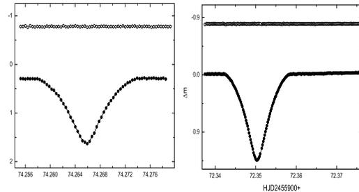
**Figure 3:** Light curves of NSVS07826147. Left panel: Eclipsing profiles of NSVS07826147 obtained with 85-cm telescope on May 26, 2012 in R band. Right panel: Obtained with 2.4-m telescope on Feb. 14, 2012 without filters. Dots refer to the magnitude differences between the target and the comparison star, and open circles to the magnitude differences between the comparison and check star.
