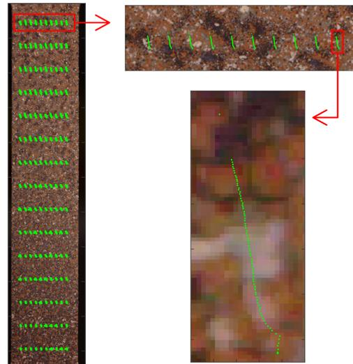
FIGURE 4. Detail of the displacement of a point during measurement.
