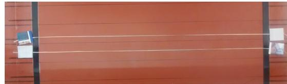
FIGURE 2. Typical yarns sample with sandwich type endings.
