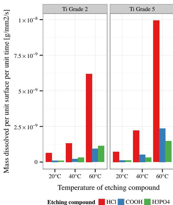
FIGURE 4. Mass dissolution per unit time of Ti grade 2 and Ti grade 5 in each etching compound.
