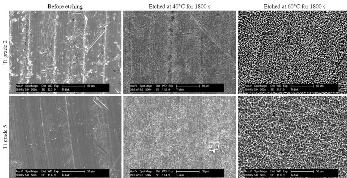
FIGURE 3. SEM images of grade 2 and grade 5 titanium discs before etching and after etching in HCl at 40°C and 60°C for 1800 seconds.
