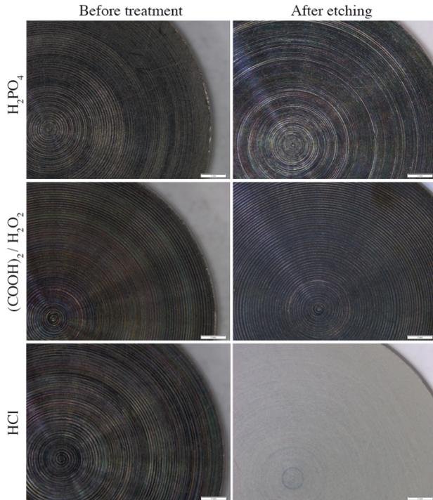
FIGURE 1. Stereo microscopic images of titanium discs before and after etching in  $\text{H}_3\text{PO}_4$ , in the compound of  $(\text{COOH})_2 \times 2\text{H}_2\text{O}$  and  $\text{H}_2\text{O}_2$  and in 30% HCl.
