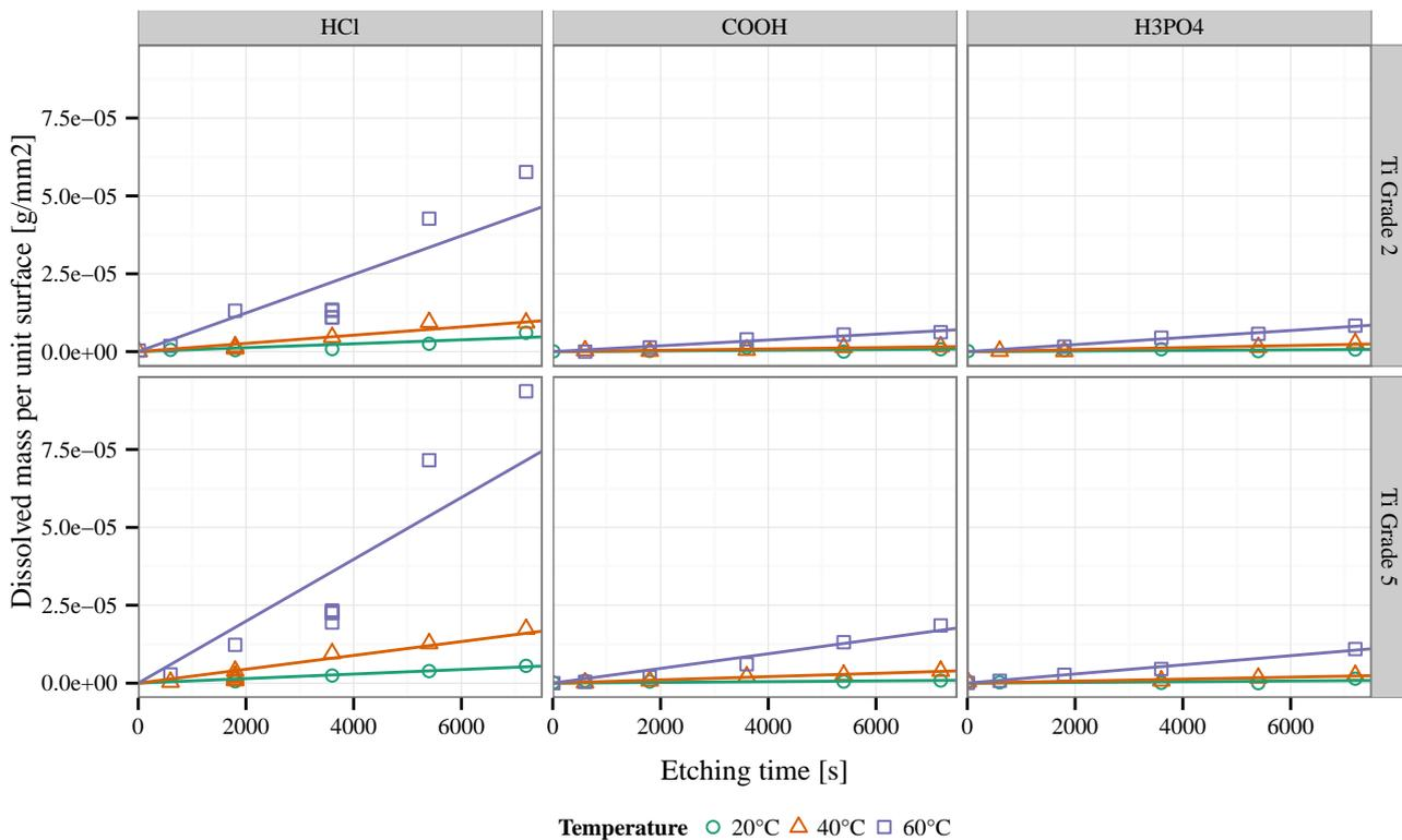
FIGURE 5. Dissolution profiles of Ti grade 2 and Ti grade 5 discs in 85%  $\text{H}_3\text{PO}_4$ , in the compound of 30%  $(\text{COOH})_2 \times 2\text{H}_2\text{O}$  and 30%  $\text{H}_2\text{O}_2$  and 30%  $\text{HCl}$  at temperatures of 20°C, 40°C and 60°C.
