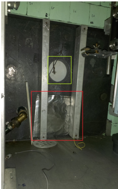
FIGURE 6. The neutron image plate (in the red frame) located in the default position below the enter of the BNCT horizontal channel (green frame).
