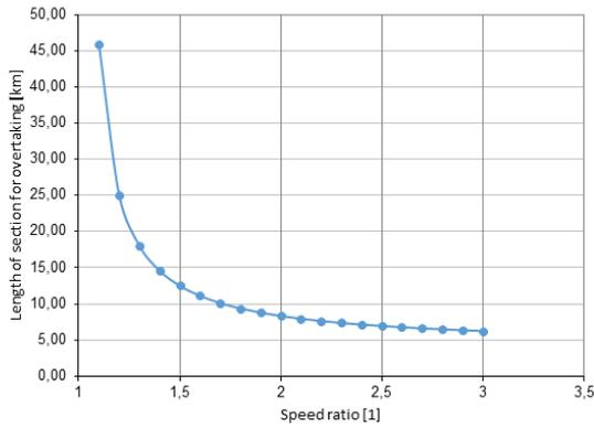
FIGURE 3. Relationship between speed ration and Length of section for overtaking.
