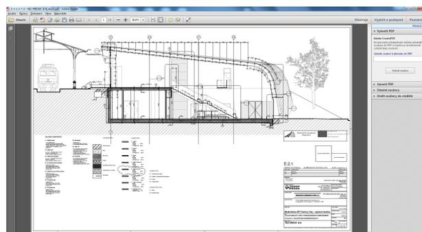
FIGURE 5. The modernization of the railway station of Karlovy Vary - station building, a cross-section B-B, Project (14-217.240) [5]
