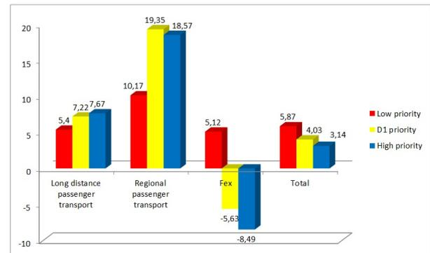
FIGURE 2. Average delay increment for different variants of Fex train priority.
