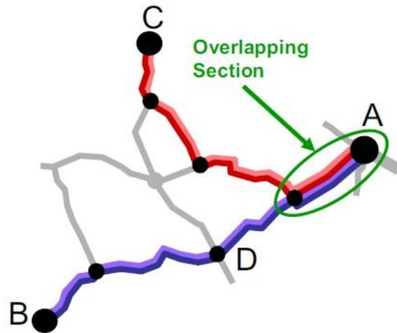
FIGURE 1. Overlapping train path line sections [4]
