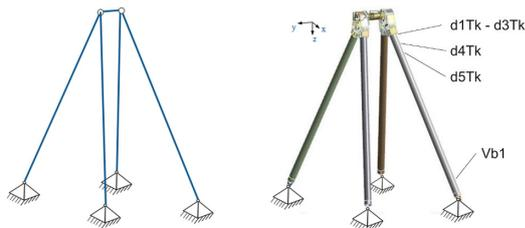
FIGURE 6. Bar- and 3D-FE-Model Model incl. sensor positions
