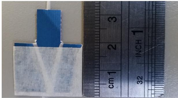
FIGURE 1. Sandwich-type terminals.
