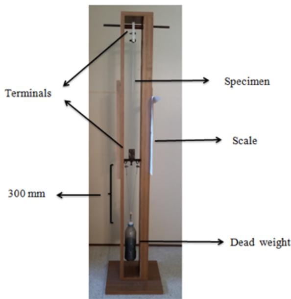
FIGURE 2. Impact testing device.
