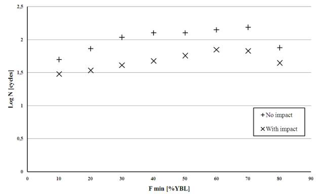
FIGURE 3. Cycles up to failure versus load ranges: superposed results.
