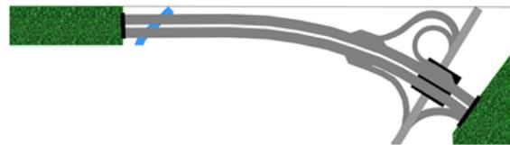
FIGURE 4. Highway section with a trumpet-type interchange.
