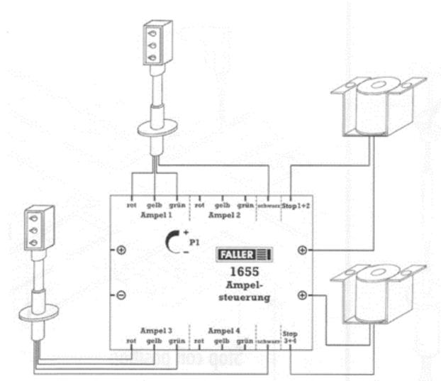
FIGURE 11. Example of intersection control. Source: [6].
