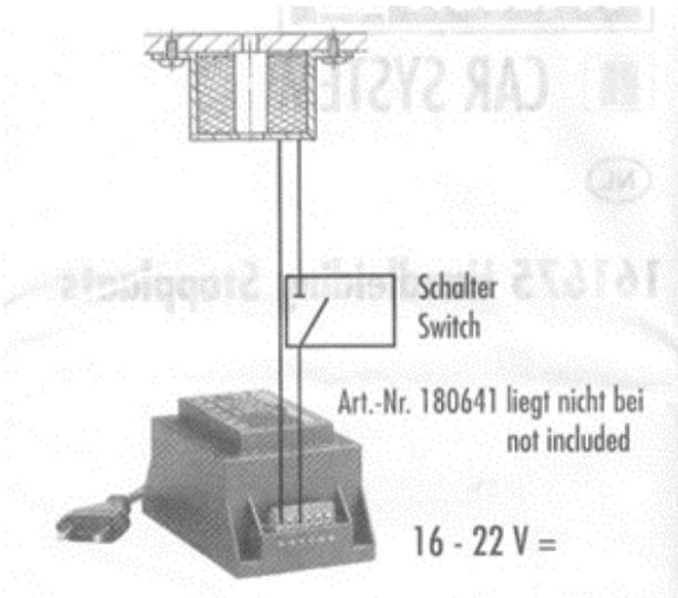
FIGURE 10. Stop section. Source: [6].
