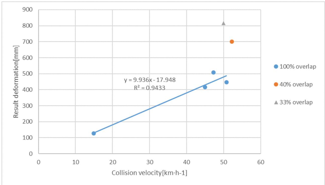
FIGURE 1. Dependency of the deformation of the vehicle from collision velocity.
