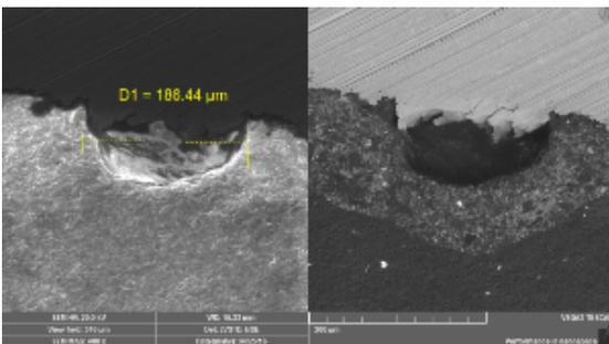
FIGURE 3. Rupture in the site of the metal-ceramic material contact.
