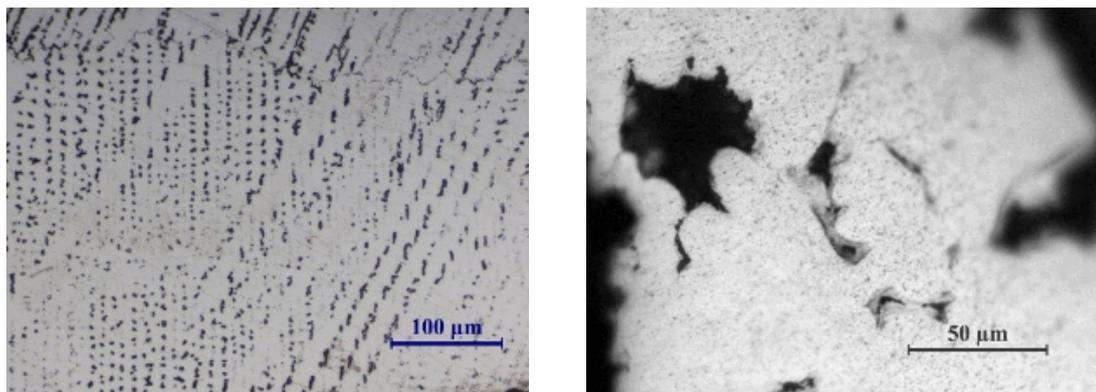
FIGURE 5. Microstructure of Co-Cr alloy .
