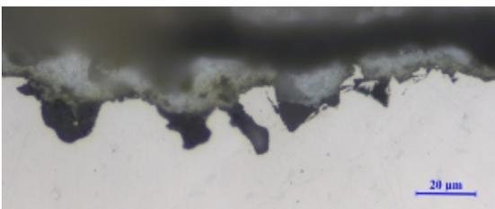
FIGURE 4. Penetration of ceramic material.
