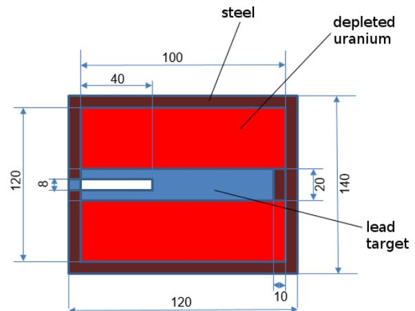
FIGURE 3. B-URAN sectional view, lead target [8]
