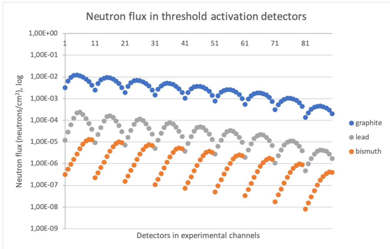
FIGURE 6. Comparison of several targets, neutron flux (neutrons/cm<sup>2</sup>), 9 sets of detectors in experimental channels (calculated by MCNP)
