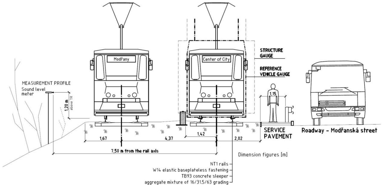
FIGURE 4. Characteristic section at the point of the noise-absorbing screen placement.
