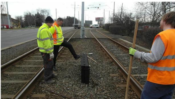
FIGURE 3. Mounting of MNAS prototypes – Vandal resistance test.
