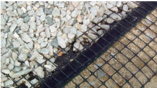
FIGURE 1. Reinforced geogrid Tensor SS.
