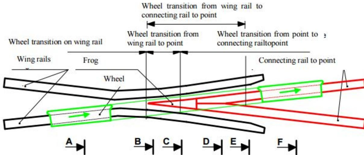
FIGURE 1. Schematic representation of the wheel set crossing over the frog – view from above [2].
