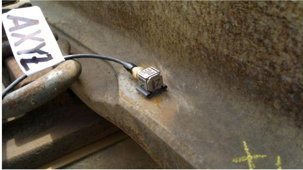
FIGURE 4. The three-axis accelerometer placed on flange of the wing rail.
