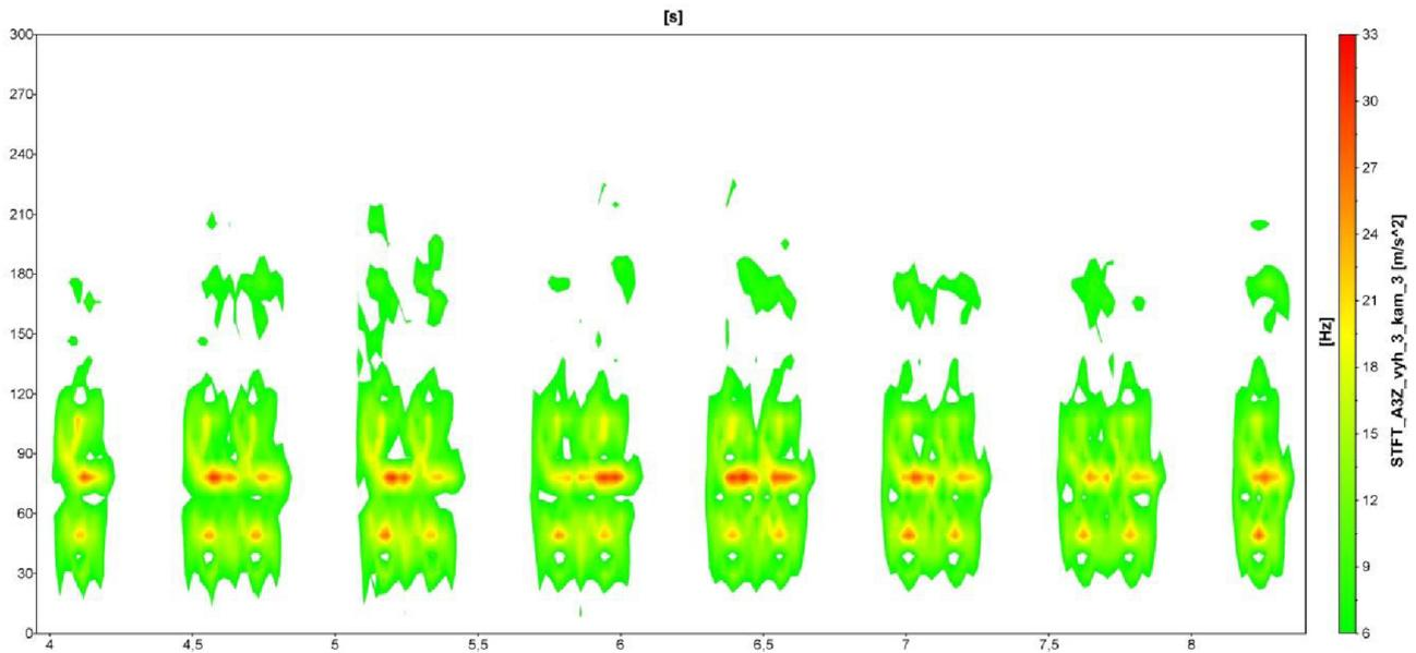
FIGURE 5. Time-frequency spectrogram calculated by STFT method, turnout no. 3, Pendolino train, third measurement campaign.
