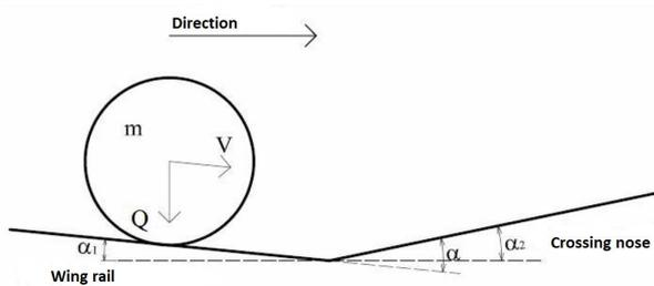
FIGURE 2. Simplified model of wheel movement through the crossing part [3].
