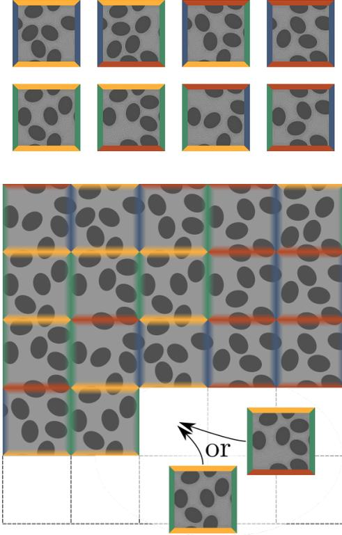
FIGURE 1. The compressed microstructural geometry represented with the set of Wang tiles (top) and an illustration of a step in the tiling algorithm with partially assembled microstructure (bottom).
