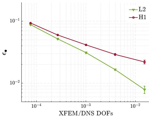
FIGURE 4. Convergence of  $L_2$  and  $H_1$  errors with increasing number of DOFs in the coarse discretization.
