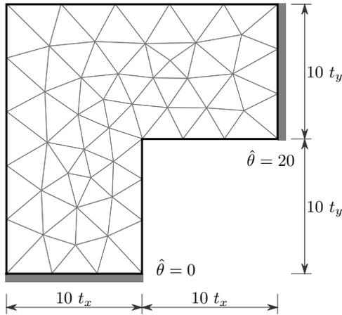
FIGURE 3. A scheme of the problem definition. The edge lengths  $t_x$  and  $t_y$  of the tiles were set as  $t_x = t_y = 6$ . All quantities are in consistent units.
