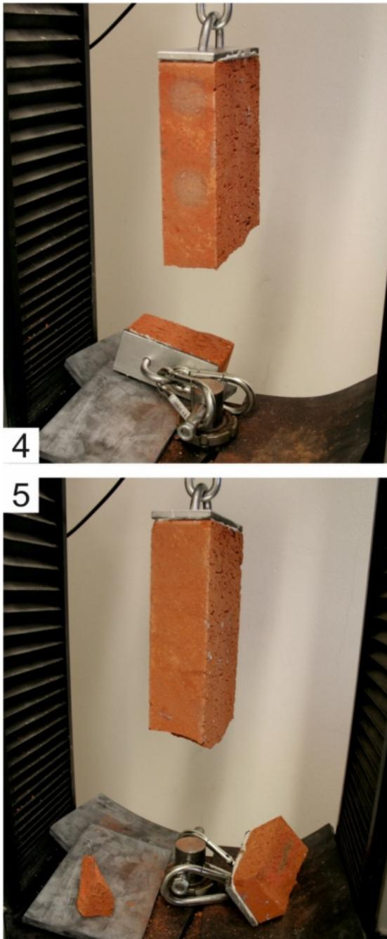
FIGURE 2. Failure of specimens no. 4 and 5.
