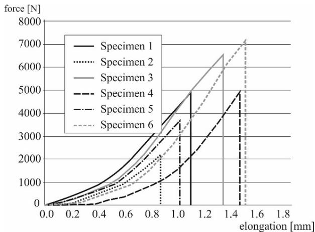
FIGURE 5. Working diagram force-elongation of bricks.
