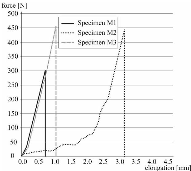
FIGURE 10. Working diagram force-elongation of mortar.
