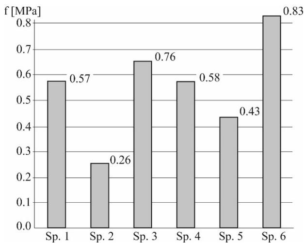
FIGURE 6. Tensile strength of bricks.
