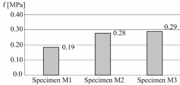
FIGURE 11. Tensile strength of mortar.
