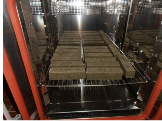
FIGURE 3. Specimens in the climatic chamber.
