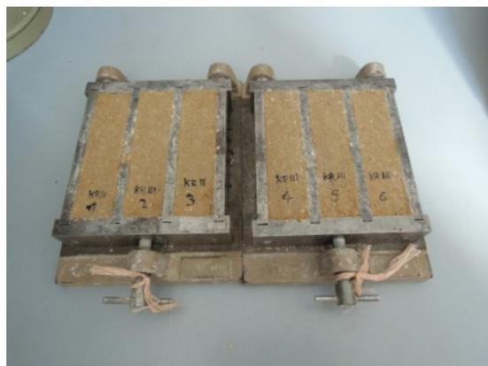
FIGURE 3. Production of the test bodies.
