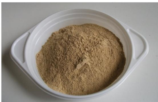
FIGURE 2. Illitic-kaolinitic clay.
