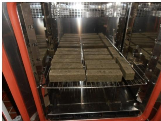
FIGURE 4. Test bodies in the air-conditioning chamber.
