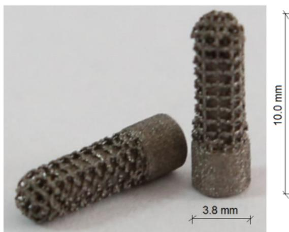
FIGURE 8. Whole implant body of the implant for further research. Implant has a homogeneous stem and an outer layer comprising of the trabecular structure. The implant has been patented in Czech Republic [6].
