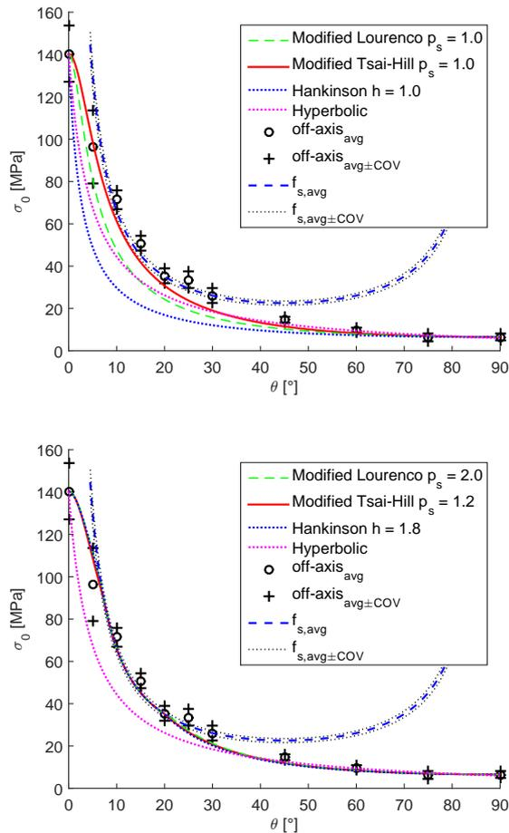
FIGURE 1. The experimental data of Sitka spruce [7] with uncalibrated (top) and calibrated (bottom) failure conditions.
