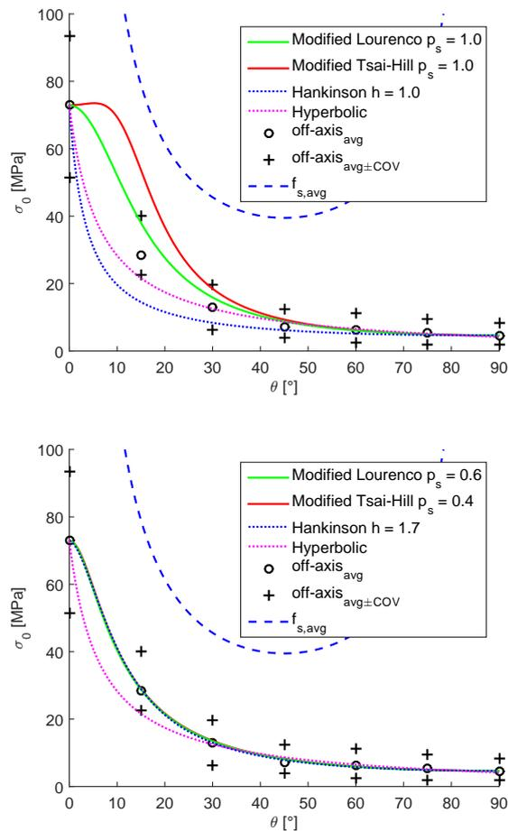
FIGURE 5. The experimental data of Cupiúba [20] with uncalibrated (top) and calibrated (bottom) failure conditions.
