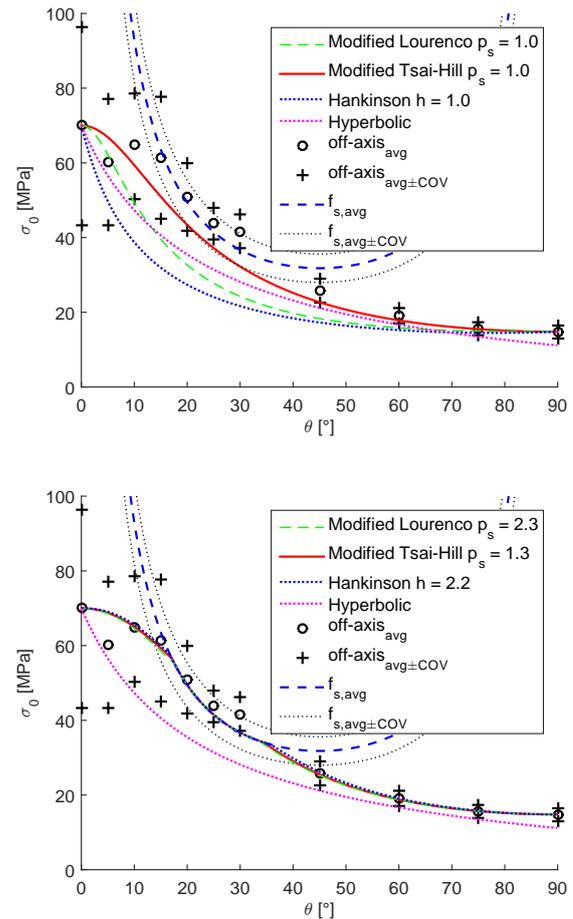
FIGURE 2. The experimental data of Katsura [7] with uncalibrated (top) and calibrated (bottom) failure conditions.
