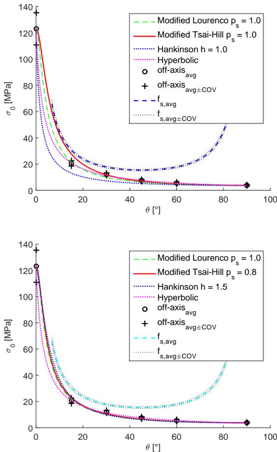
FIGURE 3. The experimental data of Douglas fir [18] with uncalibrated (top) and calibrated (bottom) failure conditions.
