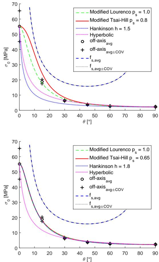
FIGURE 4. The experimental data of Douglas fir laminated veneer [19] with uncalibrated (top) and calibrated (bottom) failure conditions.
