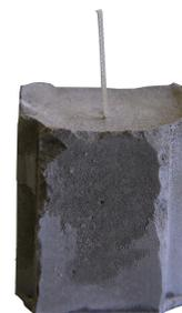
FIGURE 2. Cement specimen with single fiber for pullout tests.
