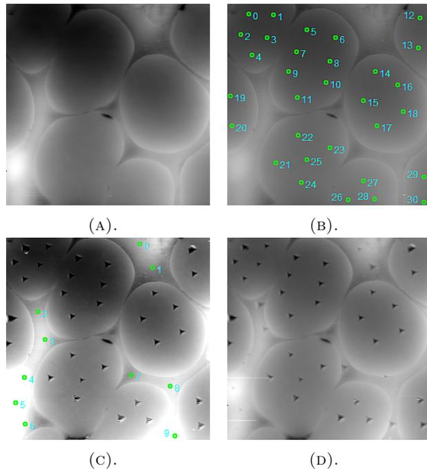
FIGURE 1. Indentation steps in longitudinal direction.
