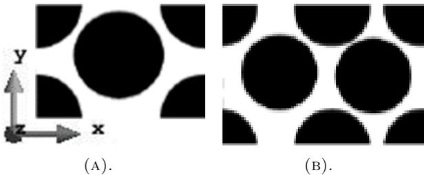
FIGURE 4. Microscale level of yarn, (A) two-fiber SEPUC-1, (B) four-fiber SEPUC-2.
