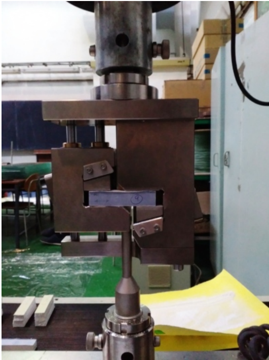
FIGURE 4. Test of shear strength perpendicular to the plate plane according to ASTM D5379.
