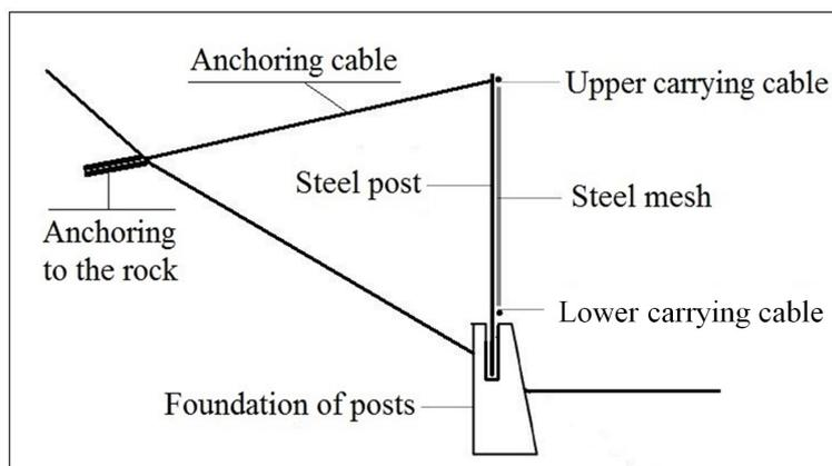
FIGURE 8. Protective fence – schematic cross section.
