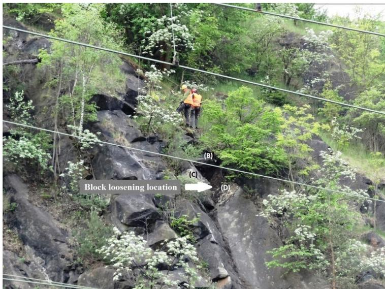
FIGURE 4. The location of a loosening of the fallen rock block.
