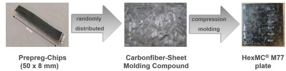
FIGURE 2. C-SMC production process (reprinted from [6])
