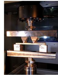
FIGURE 7. Mode II testing setup
