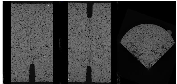
FIGURE 4. Visualization of damaged sample in three perpendicular planes based on the reconstructed micro-CT data corresponding to displacement  $320\ \mu\text{m}$
