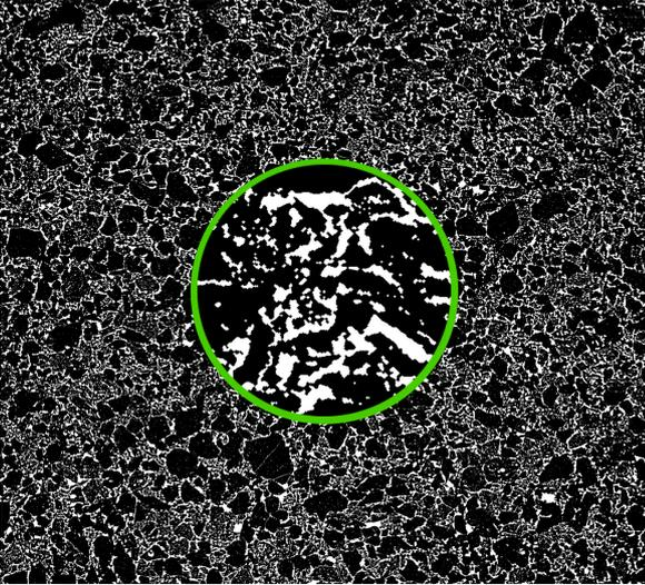
FIGURE 5. Result of improper segmentation in grey-intensity space leading to substantial loss of information with upscaled detail of over-segmented structure.
