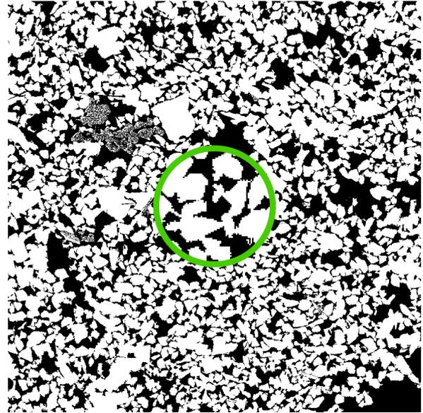
FIGURE 6. Output from segmentation procedure showing image suitable for structural analysis with highlighted detail of microstructure.
