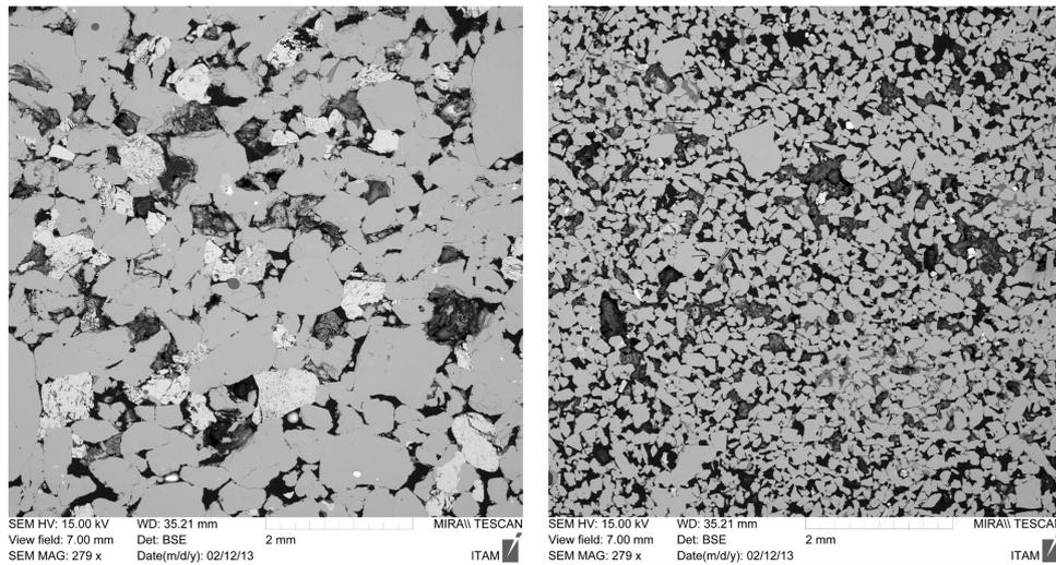
FIGURE 4. Arkose from the Charles Bridge (left) and Petřín sandstone (right) captured using BSE detector in SEM.
