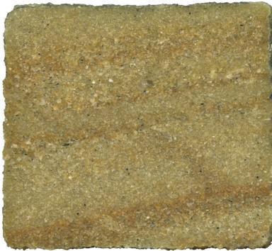
FIGURE 2. Nehvizdy sandstone sample captured using high-resolution flatbed scanner.
