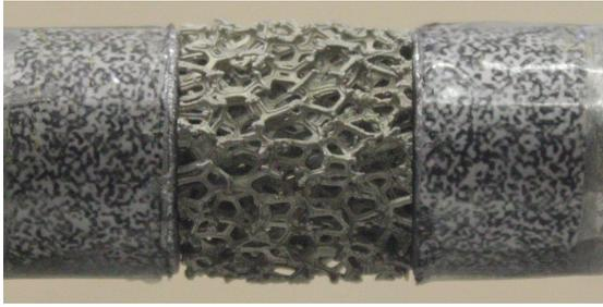
FIGURE 1. Ni/PU foam specimen in the SHPB experimental setup
