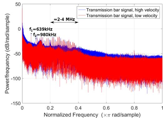
FIGURE 7. Periodogram of incident signal:  $l_s = 500$  mm (long striker),  $v_s = 45.21$   $\text{ms}^{-1}$  (high striker velocity) and  $l_s = 500$  mm (long striker),  $v_s = 21.03$   $\text{ms}^{-1}$  (low striker velocity)
