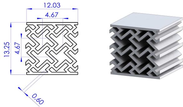
FIGURE 3. 2D missing-rib auxetic structure
