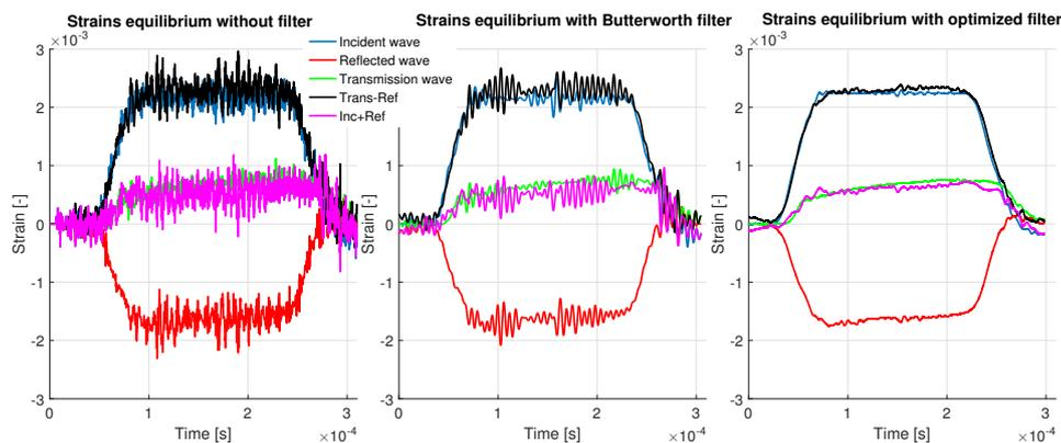
FIGURE 10. Comparison of strain equilibrium obtained without signal filtering and with two different filters:  $l_s = 500$  mm (long striker),  $v_s = 24.05$  ms<sup>-1</sup> (high striker velocity)
