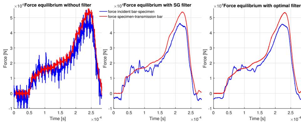
FIGURE 9. Comparison of force equilibrium obtained without signal filtering and with two different filters:  $l_s = 500$  mm (long striker),  $v_s = 45.36$  ms<sup>-1</sup> (high striker velocity)
