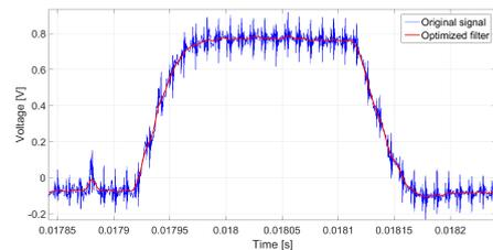
FIGURE 4. Elastic wave signal with applied filter
