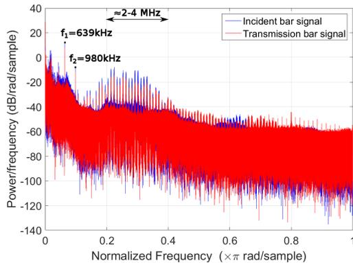
FIGURE 5. Periodogram of incident and transmission signal:  $l_s = 500$  mm (long striker),  $v_s = 20.85$   $\text{ms}^{-1}$  (low striker velocity)
