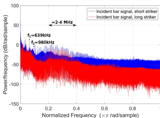
FIGURE 6. Periodogram of incident signal:  $l_s = 500$  mm (long striker),  $v_s = 24.05$   $\text{ms}^{-1}$  (low striker velocity) and  $l_s = 100$  mm (short striker),  $v_s = 19.32$   $\text{ms}^{-1}$  (low striker velocity)
