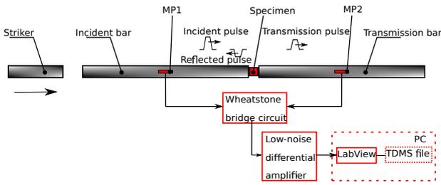
FIGURE 1. Basic scheme of SHPB
