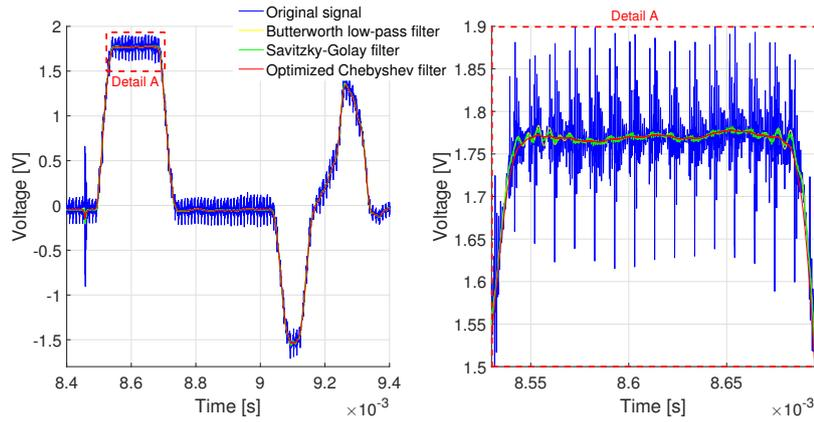
FIGURE 8. Comparison between different filters for incident signal:  $l_s = 500$  mm (long striker),  $v_s = 45.36$  ms<sup>-1</sup> (high striker velocity)
