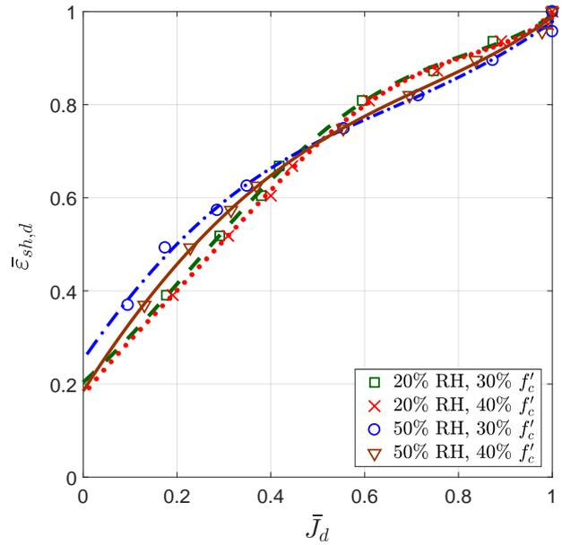
FIGURE 5. Comparison of normalized drying shrinkage and normalized drying creep evaluated from the experiments of Keeton at 20 % and 50 % relative humidity and two levels of loading.  $f'_c$  is the compressive strength at the age of loading. Points are the experimental data.
