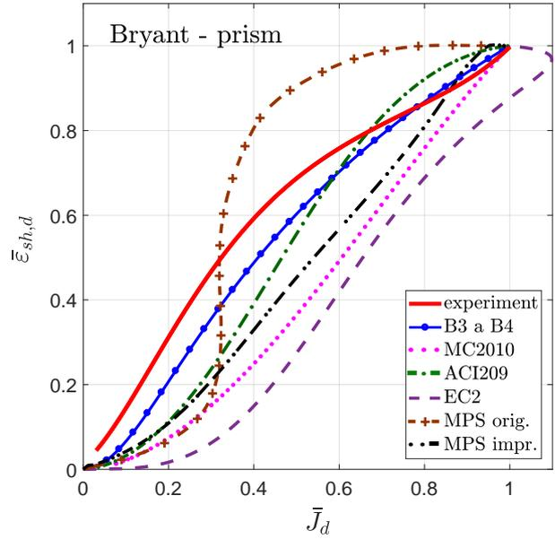
FIGURE 10. The comparison of the experimental data, prediction models and FE simulations of the Bryant's experiment,  $2V/S = 75$  mm (prism).
