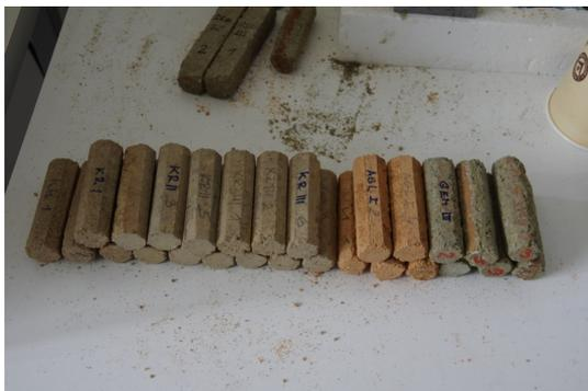
FIGURE 5. The test bodies shape of prism with octahedron base.
