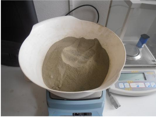
FIGURE 7. Montmorillonite clay.
