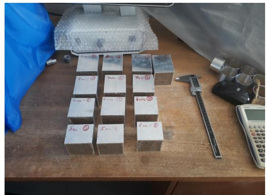
FIGURE 6. The test bodies for drying rate experiment.
