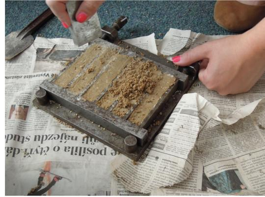
FIGURE 9. The pressing down to the mould.
