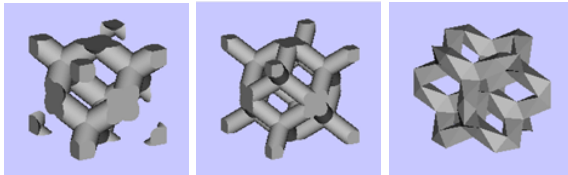
FIGURE 1. Basic element cells for creation of the test specimens.
