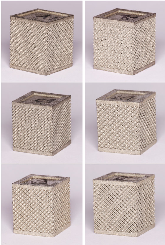
FIGURE 2. Real manufactured specimens A-F used for the uniaxial compression test.
