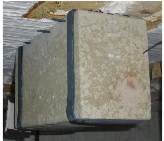
FIGURE 3. Concrete block after the fire exposure.
