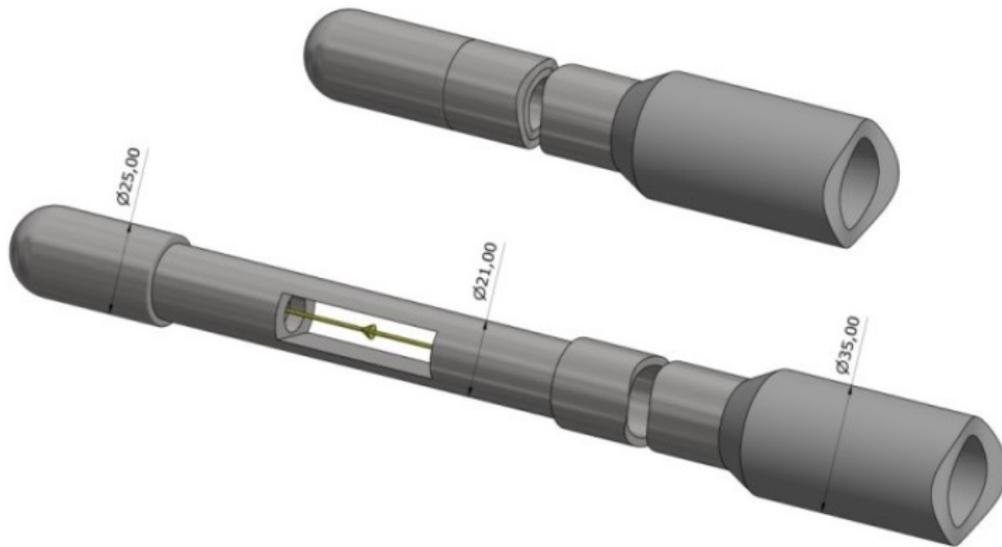
FIGURE 3. Optical probe head with open and closed measuring space.
