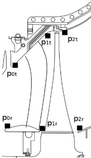
FIGURE 1. Position of static pressure taps.
