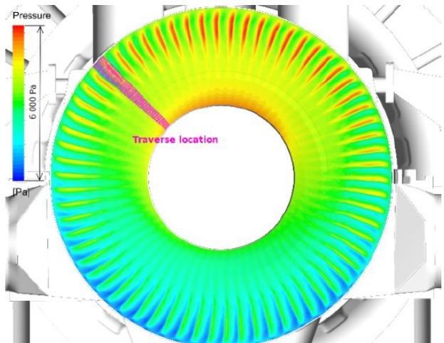
FIGURE 10. Static pressure flow field in Plane 2.
