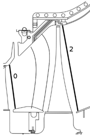
FIGURE 2. Position of traversing planes.
